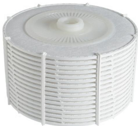
Depth filter modules make it possible to handle large filter areas in a simple manner and have been used in various food & beverage applications for many years. Filtration with such modules is carried out in an enclosed system (DISCSTAR™). The filter medium used in lenticular modules is a depth filter sheet. A combination of surface,
