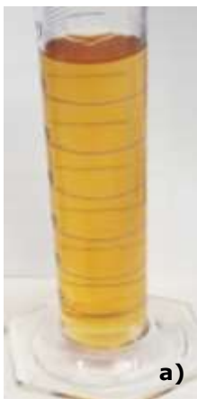
Picture 3: API after surface filtration (a, stirred-up) and after CARBOFIL™ CA treatment (b).
