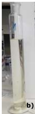
Picture 3: API after surface filtration (a, stirred-up) and after CARBOFIL™ CA treatment (b).
