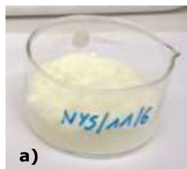
Picture 4: Resulted API powder after filtration with CARBOFIL™ CA and crystallisation. 0.55 cm 2 (a) and 1.1 cm 2 (b) activated carbon per gram product was used.
