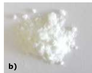
Picture 4: Resulted API powder after filtration with CARBOFIL™ CA and crystallisation. 0.55 cm 2 (a) and 1.1 cm 2 (b) activated carbon per gram product was used.
