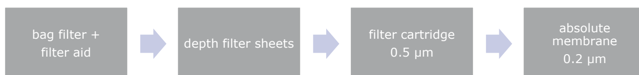
Figure 1: Former process with a total of 4 filtration steps
