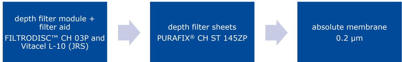
Figure 2: New process with FILTRIX products
