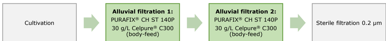
Figure 8: Optimized clarification process of a mAb-producing CHO cell culture suspension. A double-stage filtration was necessary to reduce the initial turbidity of >2000 NTU to less than 30 NTU.
