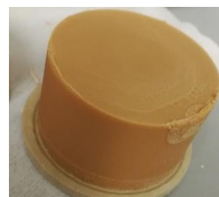
Figure 4: Filter cake generated in trial 8.1. The cells have settled between the DE particles, allowing the liquid to flow through the cake.
