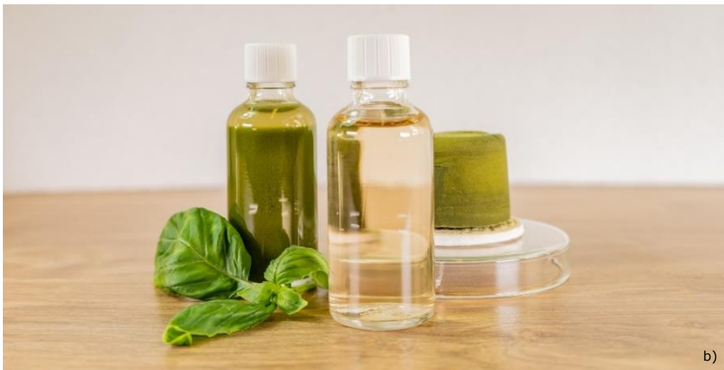
Figure 6: Basil extract – Overview of all filtrates (a) and comparison of the unfiltered extract with the filtrate from experiment 4 (b). The turbidity was reduced from over 1100 NTU to 0.4 NTU in experiment 4. A filter cake with a height of 3.2 cm was generated.
