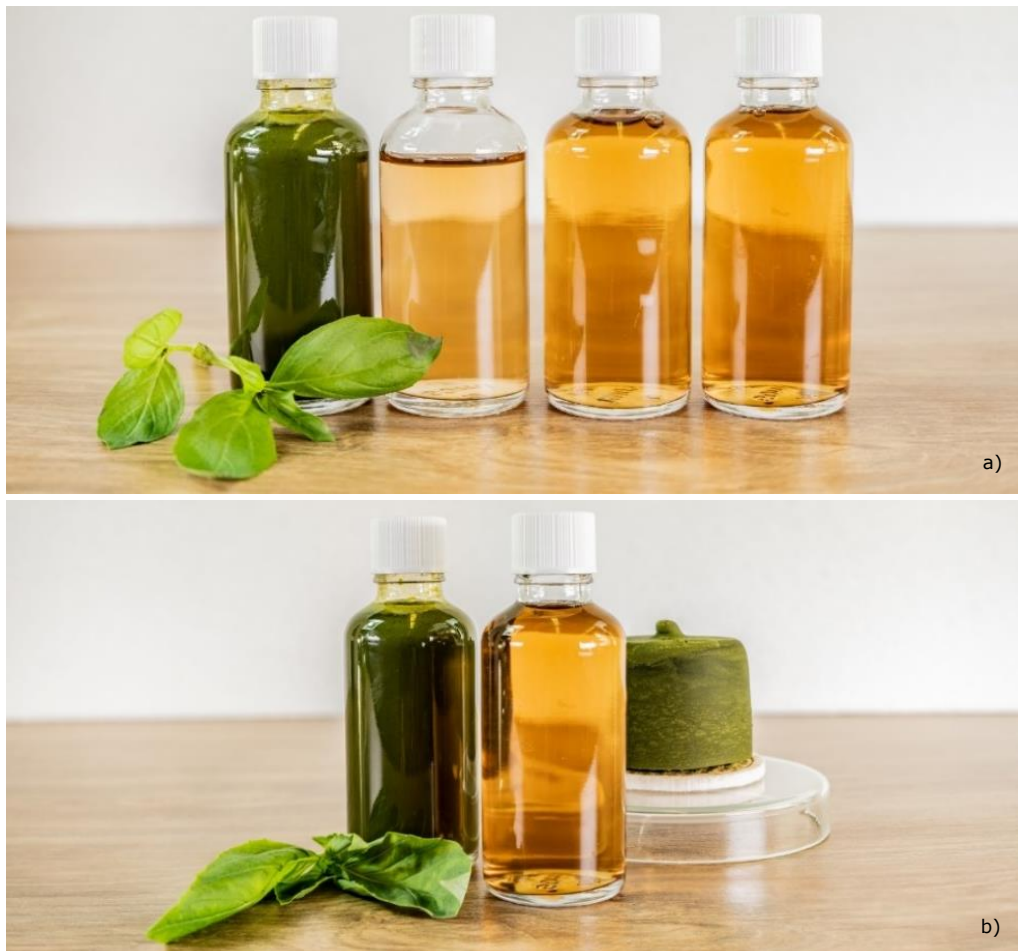
Figure 5: Thai basil extract – comparison of the filtrates from experiments V2, V3 and V4 (a) and direct comparison with the filtrate from experiment 4 (b), in each case with the unfiltered extract. Using the alluvial filtration technology, the initial turbidity of 1460 NTU could be reduced to around 2 NTU and lower (experiments 2, 3 and 4). Since very little filtrate was generated in the first experiment, it is not shown here.
