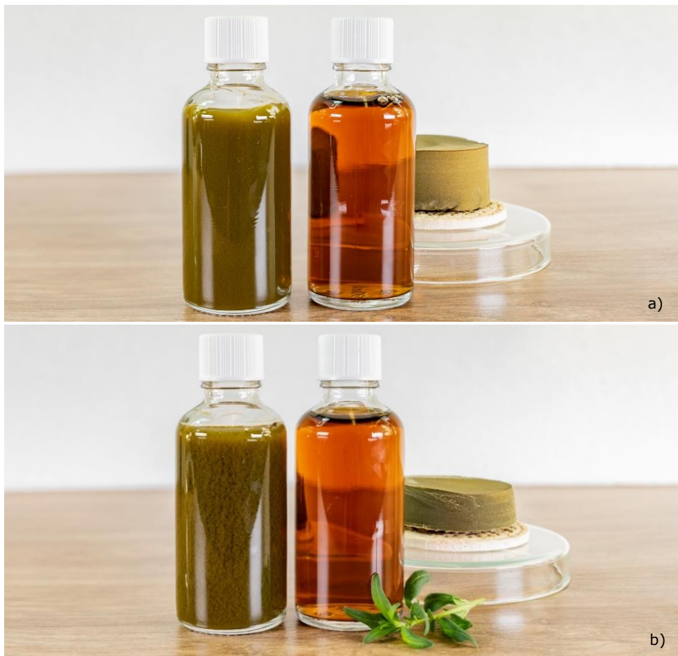
Figure 3: Ysop extract – unfiltered and filtered extract from experiments 2 (a) and 3 (b). The unfiltered extract is compared with the filtrate and the filter cake generated. Since twice the amount of diatomaceous earth was used in the second experiment, a significantly higher filter cake resulted - compared to experiment 3.
