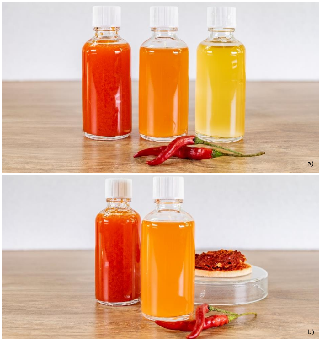
Figure 7: Chili extract – Overview of the filtrates (a) and comparison of the unfiltered filtrate with the filtrate from filtration experiment 1 (b). Although no filter aid was added to the unfiltered chili extract, a filter cake was built up in each case. However, due to the very large chili seeds, this was formed very irregular.
