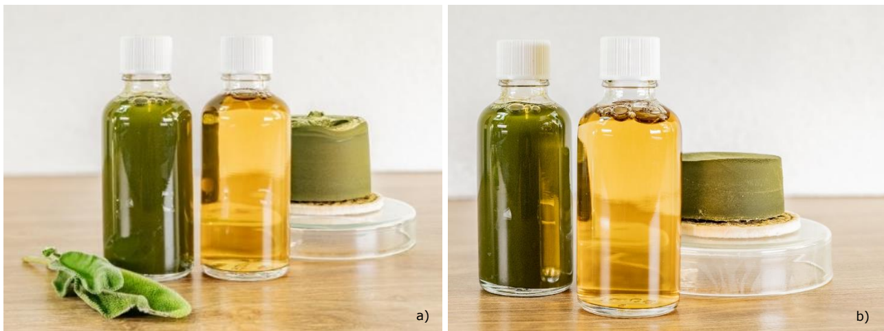
Figure 4: Sage extract – filtration experiment 4 (a) and 5 (b). The unfiltrate is compared with the filtrate in each case. The filter cakes generated in the process are also shown and differ in height – depending on the volume filtered in each case as well as the amount of diatomaceous earth added. In the fourth experiment, 880 mL of extract was filtered, resulting in a filter cake of 3.5 cm (a).
