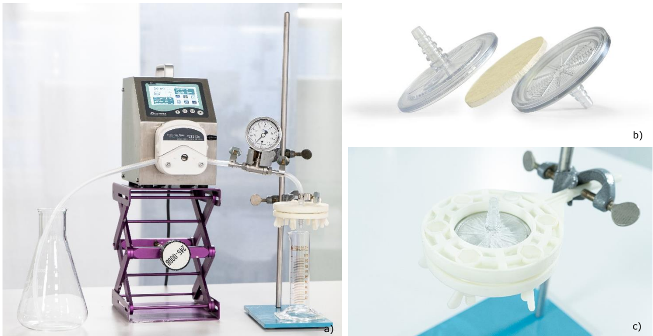
Figure 5: Overview of the experimental setup and the individual parts of the filter capsule used. The experimental setup (a) consisted of a peristaltic pump, a pressure gauge and the filter capsule. Any filter sheet is placed between the individual parts of the Mini Capsule (b) and then sealed with the synthetic holder (c). Since yeast cells settled rapidly, the unfiltered suspension was continuously mixed using a magnetic stirrer. The filtrate was collected in a graduated cylinder each time to determine the filtered volume over time.
